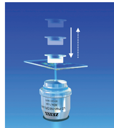
Pick-up LCM via AdhesiveCap Touch
