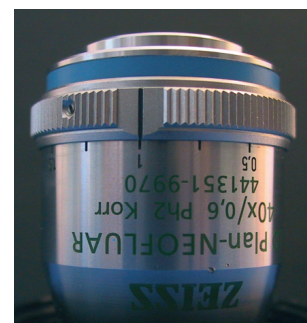
FrameSlide => between dot and 0, Regular glass slide (1 mm thick) => 1.
